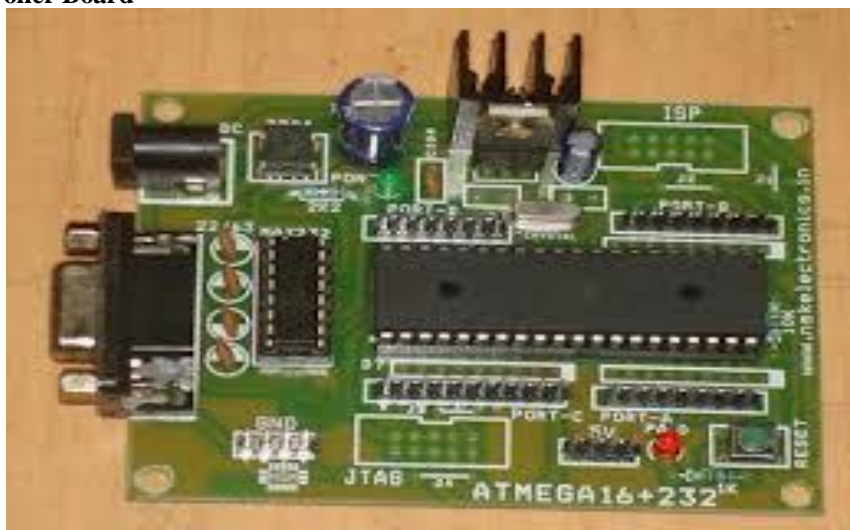
Figure 7 AVR development board with ATMEGA 32 Controller
