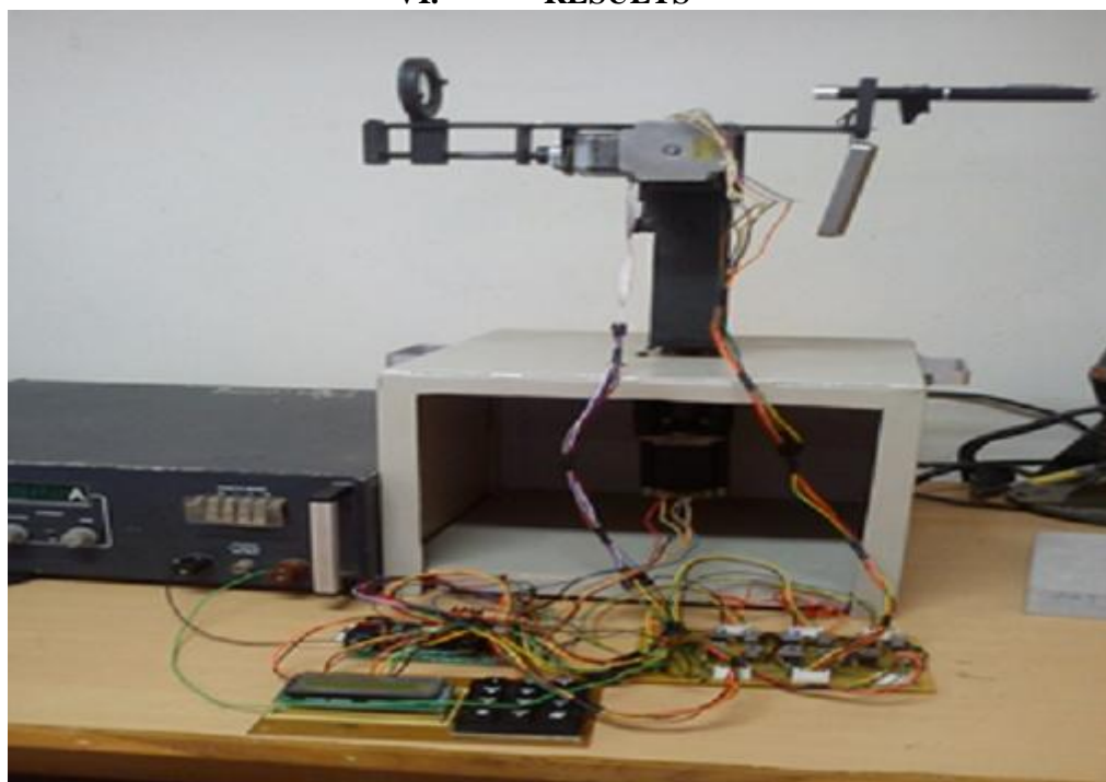
Figure 12 Experimental setup of Laser based guidance system for projectile
